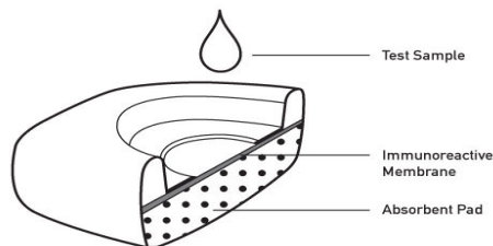
Figure 1: MedMira's Rapid Flow-Through Technology Platform
